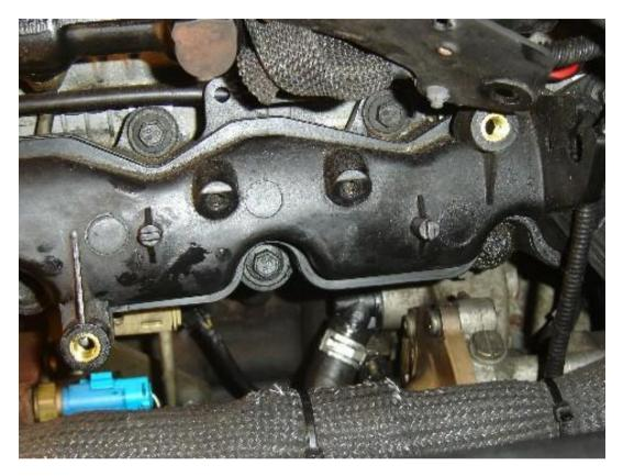
Now using a long pair of pliers squeeze together and release the clip then pull off the hose. You will loose some coolant at this point. Now you can see the bolt that holds the stat to the water pump.
