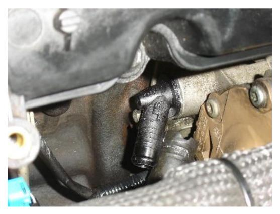
You are going to need a ¼ drive flexible ratchet to undo the bolt 'cos there isn't a lot of room to turn a tool in that space. But it is possible. I used the one in the picture below with the key used to give an idea of the size of ratchet handle needed to get in the space.
