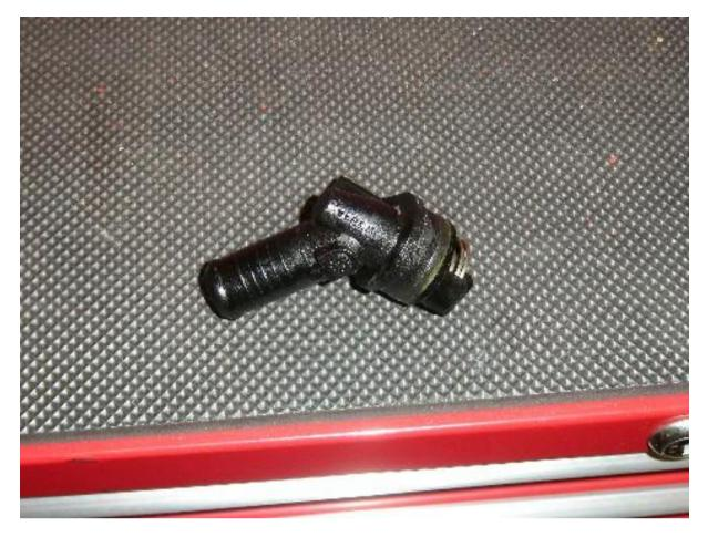
Putting it back together is simply a reversal of the above but smear the rubber 'O' ring on the new thermostat with Vaseline to make it easy to push into place.
